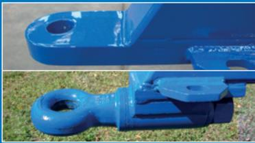
■ Standard plate tongue makes hitching up easier using the quick hitch. Optional swivel tongue is ideal for rougher country
