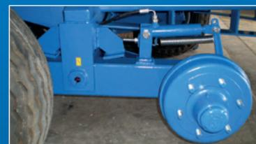
■ Hydraulic or air brakes with extra adjustable external return springs to ensure brake pad release
