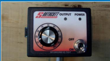
■ Electronic floor speed control mounted in tractor
