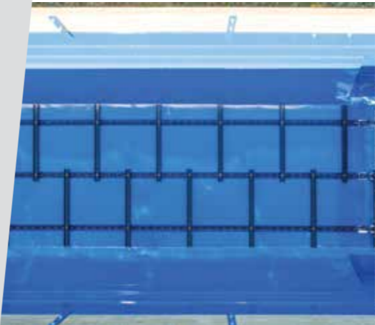
Pivoting cross conveyor with tracking strip (optional)
