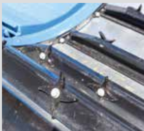
Rolling teeth keep bales moving smoothly
