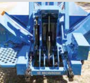
Double ram loading system
