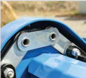
Heavy-duty 3" 12,000 lb roller chain
