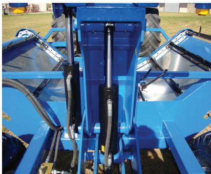
■ The double ram loading system lowers the bale gently all the way to the cradle without sudden drops which can damage feed out bars
