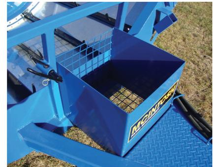
■ Steel box to hold plastic wrap. The mesh floor allows water and dirt to fall out and reduces the smell compared to an enclosed box
