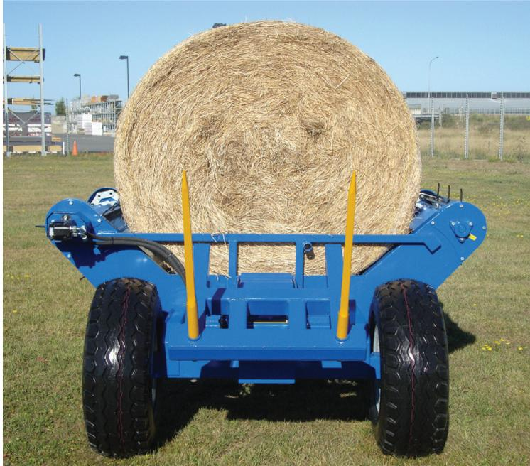
■ Axles can be adjusted to 3 widths (1620, 1720 & 1940mm) for different land conditions or to fit wider tyres. With the tyres in the above narrow position, the Bale Feeder is still very stable with this 5'3" hay bale
