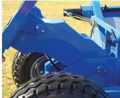
■ The large lifting arm makes the whole lifting frame very strong when travelling with a bale
