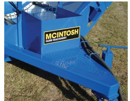
■ Checker plate to stand on when removing netting in one piece. The chassis goes through the cradle reducing the height. This greatly increases stability on hills
